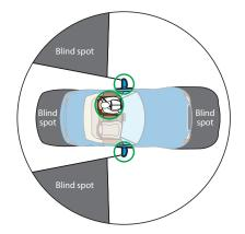
**Blind spot detectors, cameras** — Some vehicles are equipped with blind spot detectors and/or back-up cameras. While these can help you to detect hazards in blind spots or behind the vehicle, they do not replace the need to turn your head to do a shoulder check or look behind.
