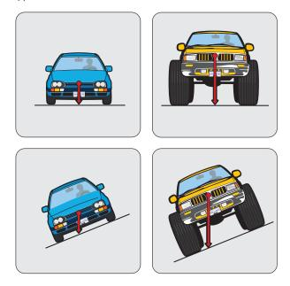
The blue car has a low centre of gravity. On a curve, the weight shifts to one side but the car remains stable. The truck, with its large wheels, has a much higher centre of gravity. On a flat surface it is stable, but when the weight shifts on a curve, the truck becomes unstable and may roll.
