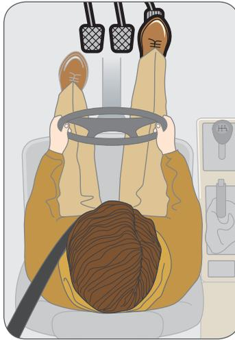
Use your right foot to operate the brake and gas pedals, and your left foot to operate the clutch. Practise doing this until you can find each pedal easily. This will help you react quickly in an emergency.
