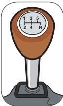
A standard transmission is always used with a clutch. The gearshift is mounted on the floor or on the steering column. Standard transmissions are built in three-, four-, five- or six-speed models. Check your owner's manual when learning to use your vehicle's gearshift.
